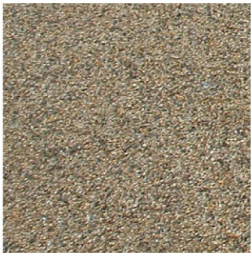
Resin bound buff coloured aggregate
