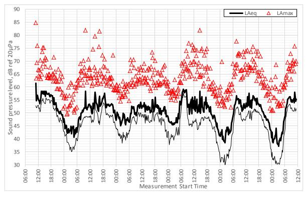
The overall sound levels at the measurement position are summarised below:
