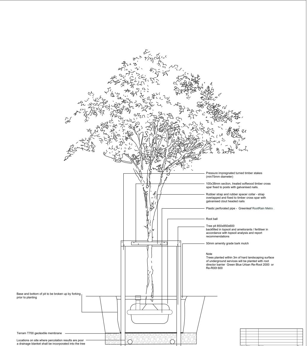
pit - incorporating 200mm depth of clean gravel or broken stone with no fines, grade 40 to 20mm with a 80mm diameter perforated plastic pipe laid around the perimeter of the pit and connected to a soakaway or drain
