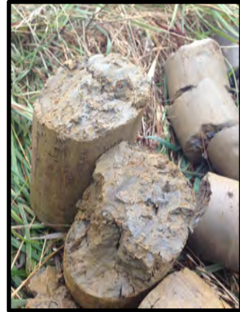
WS1 – possible shear plane at 0.85m
