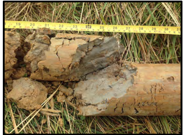
WS5 – possible shear plane at 0.65m
