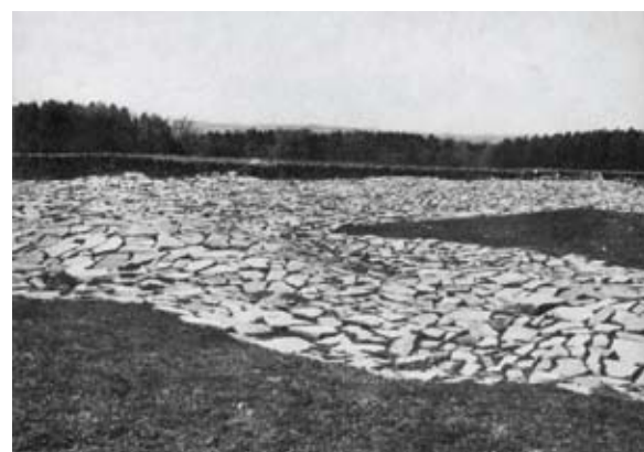
SLABS OF COTSWOLD STONE LAID OUT TO BE SPLIT BY FROST
